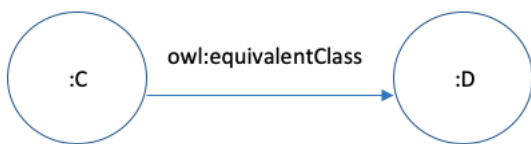
Fig. 19. RDF triplet for concept equivalence
